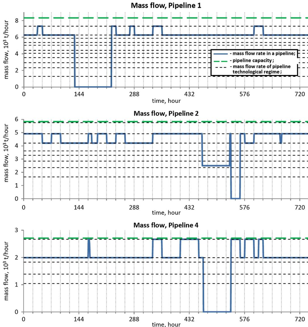
**Fig. 2.** Oil mass-flow rates in pipelines coming from suppliers.
