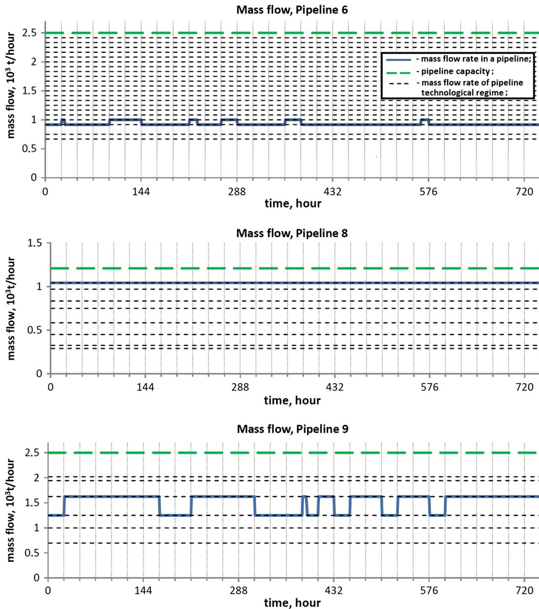
Fig. 3. Oil mass-flow rates in pipelines located between tank terminals.
