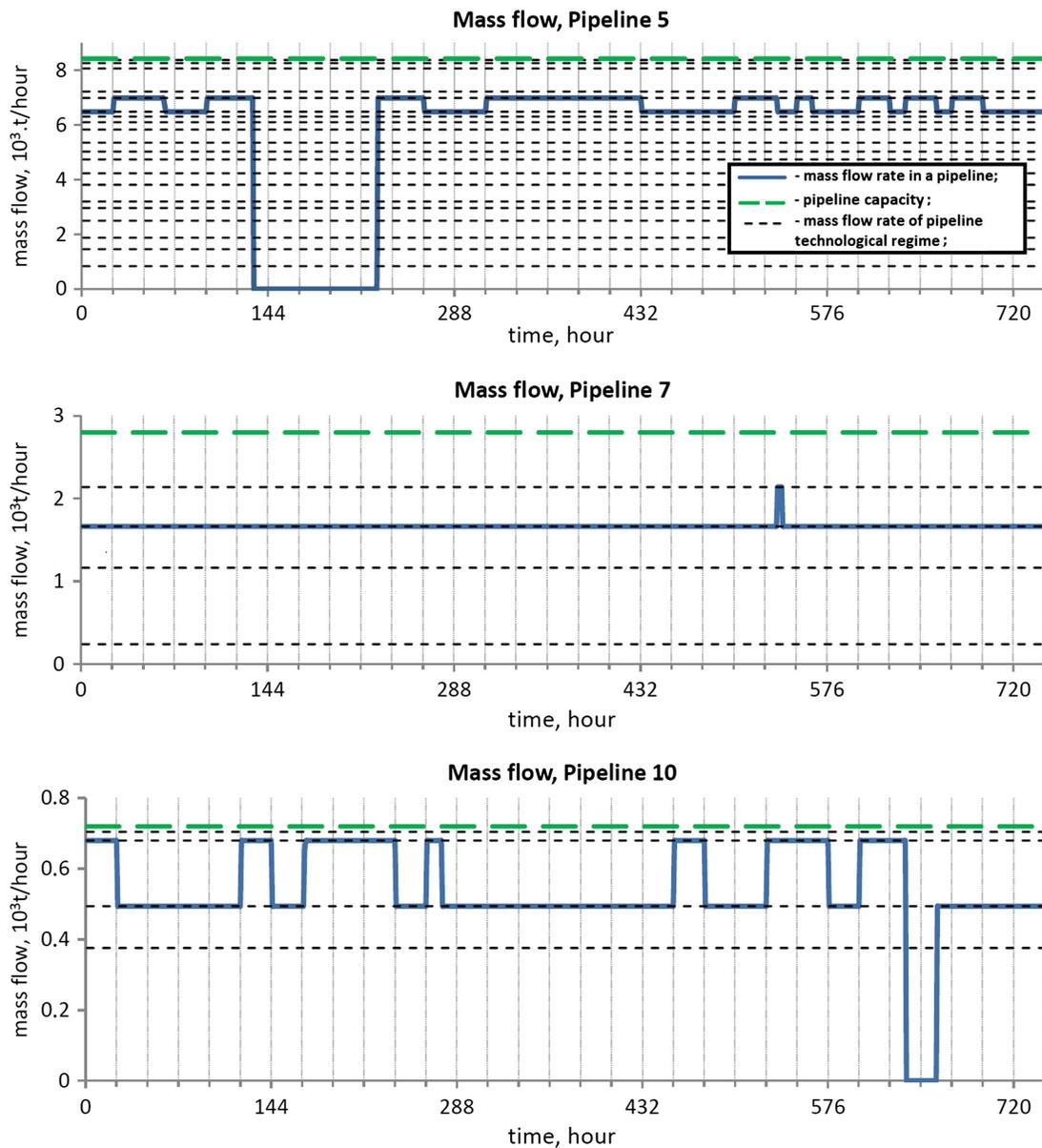
Fig. 4. Oil mass-flow rates in pipelines going to consumers.
